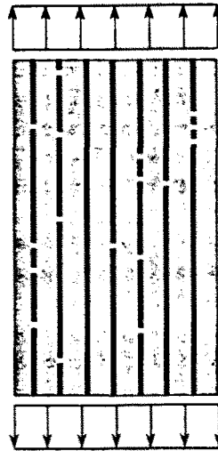
Fig. 1a. Schematic of a composite with fiber breaks.
